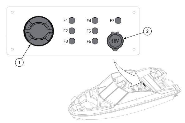
Figure 8.1 Yamarin 59 BR/SC main switch and fuse panel
