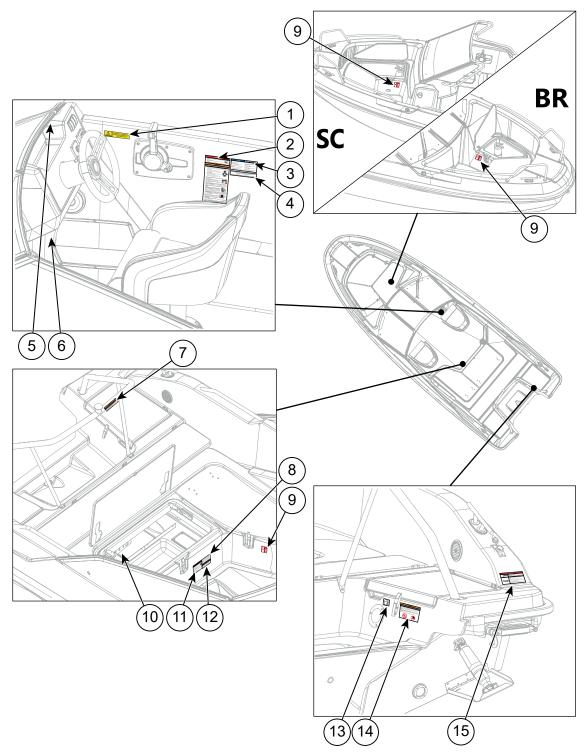
Figure 2.1 Helm station and deck safety labels
