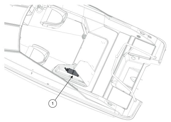
Figure 2.4 Yamarin 59 BR/SC aft deck fire extinguisher
