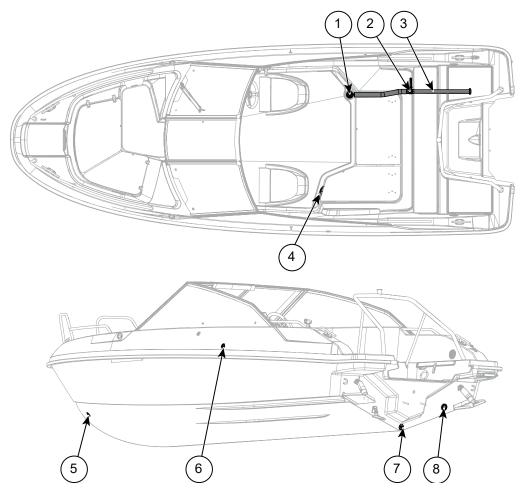
Figure 9.1 Yamarin 59 BR bilge pumps and draining
