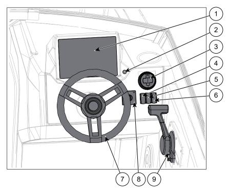
Figure 5.1 Yamarin 59 BR/SC helm station controls
