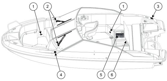
Figure 8.2 Yamarin 59 BR/SC electrical equipment
