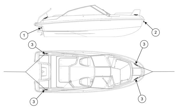
Figure 5.5 Yamarin 59 BR mooring and towing points
