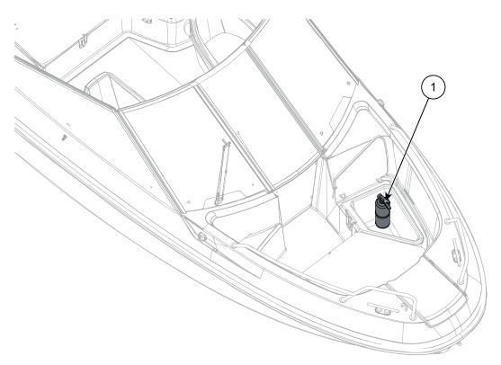
Figure 2.2 Yamarin 59 BR bow deck fire extinguisher
