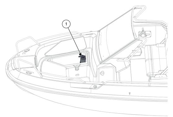
Figure 2.3 Yamarin 59 SC bow deck fire extinguisher
