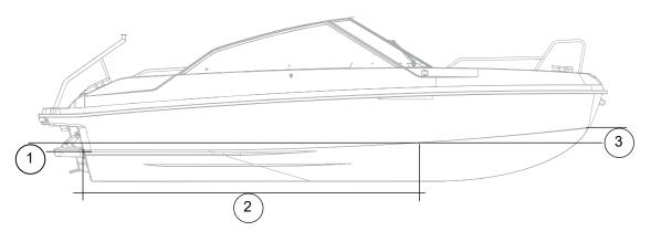
Figure 3.1 Yamarin 59 BR/SC antifouling paint area
