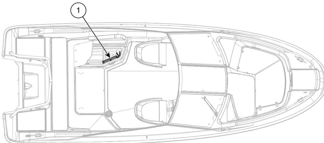
Figure 2.2 Yamarin 59 BR location of fire extinguisher
