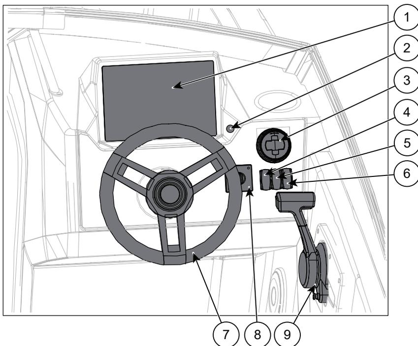
Figure 5.1 Yamarin 59 BR/SC helm station controls
