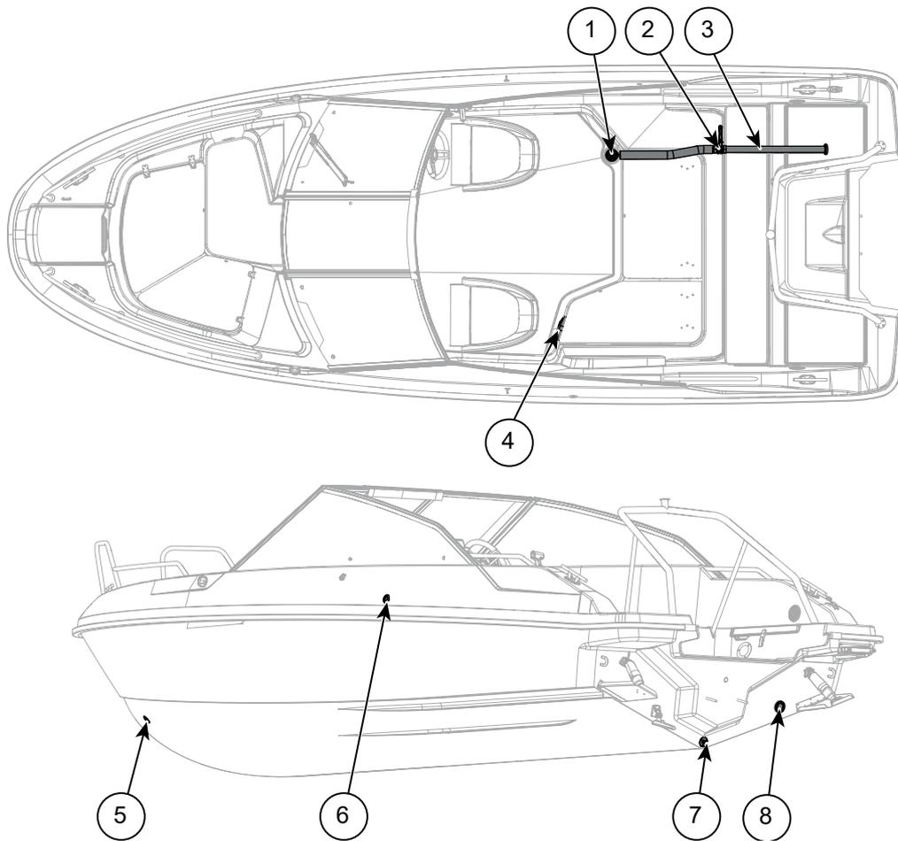
Figure 9.1 Yamarin 59 BR bilge pumps and draining
