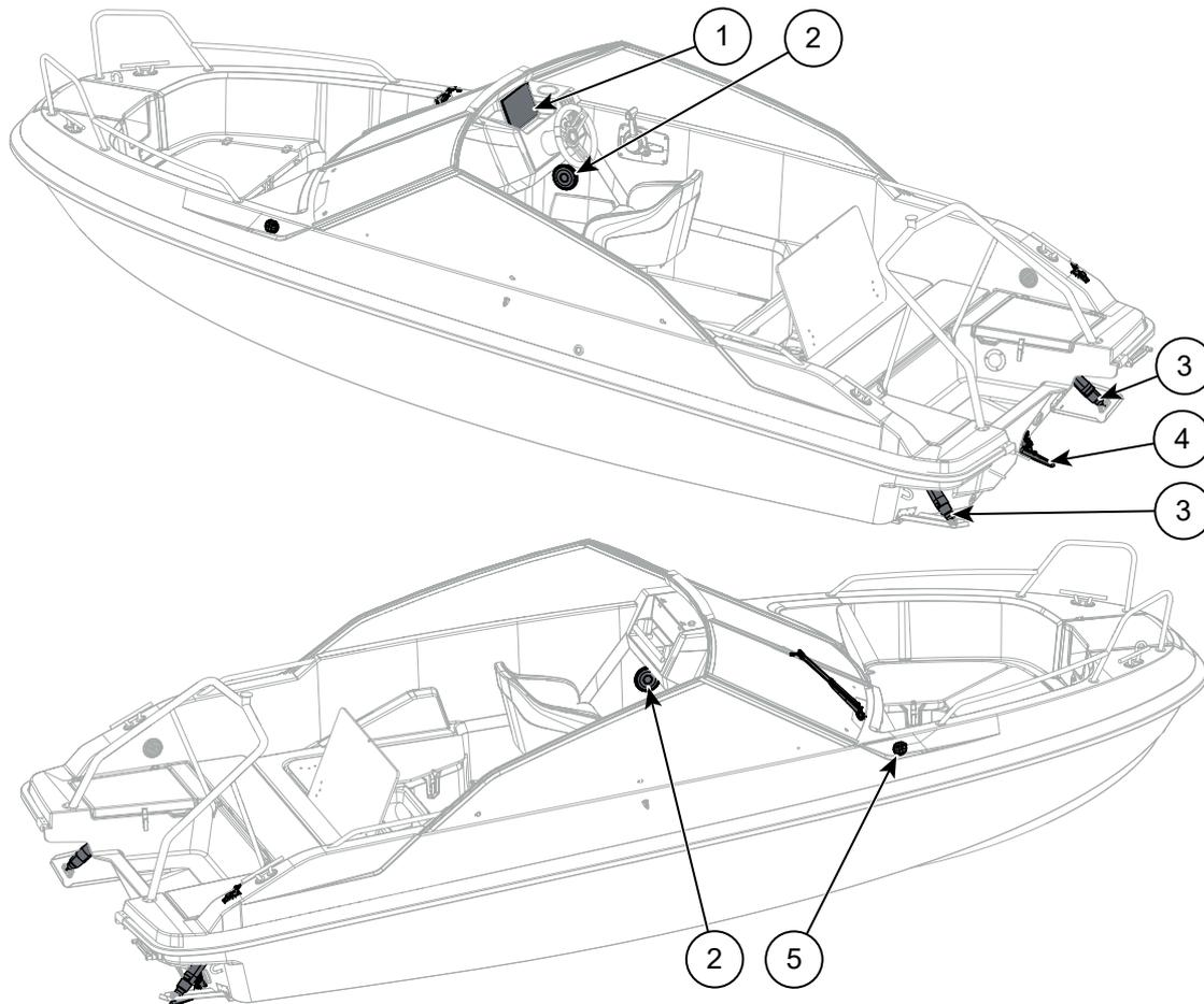
Figure 8.3 Yamarin 59 BR electrical equipment
