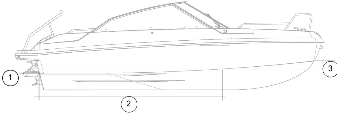
Figure 3.1 Yamarin 59 BR/SC antifouling paint area
