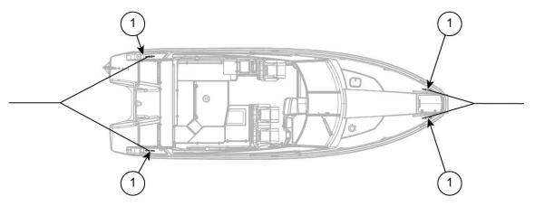
Figure 5.6 Yamarin 88 DC mooring and towing points
