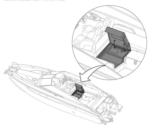
Figure 4.2 Access hatch to mid cabin
