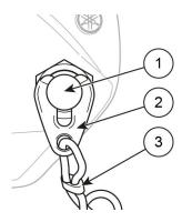
Figure 5.2 Emergency cut-off switch
