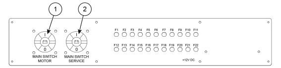
Figure 8.1 Yamarin 88 DC main switches and fuse panel
