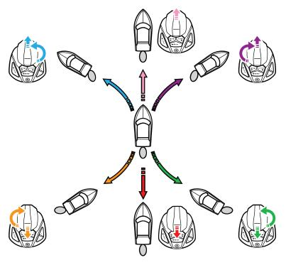
Figure 5.4 Joystick operation with a single engine boat
