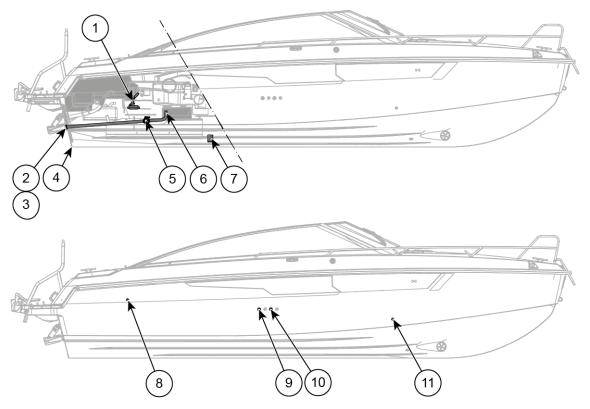
Figure 9.1 Yamarin 88 DC bilge pumps and draining
