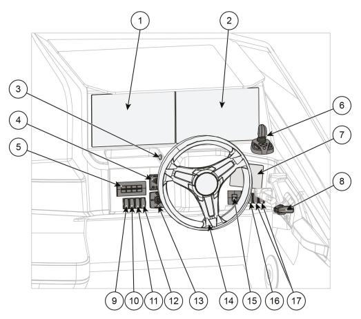
Figure 5.1 Yamarin 88 DC helm station controls
