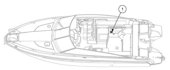
Figure 2.2 Yamarin 88 DC location of fire extinguisher
