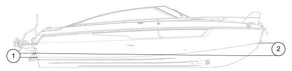
Figure 3.1 Yamarin 88 DC antifouling paint area
