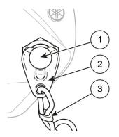
Figure 5.2 Emergency cut-off switch
