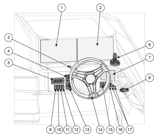
Figure 5.1 Yamarin 88 DC helm station controls
