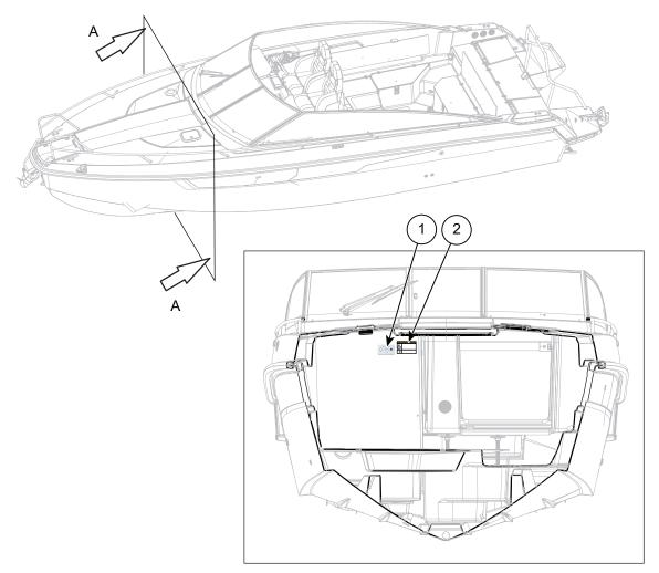
Figure 2.8 Placement of CO monitor seen from the bow
