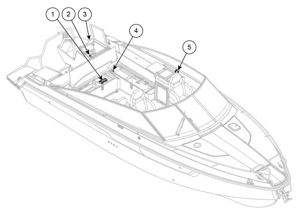
Figure 10.1 Yamarin 88 DC freshwater system
