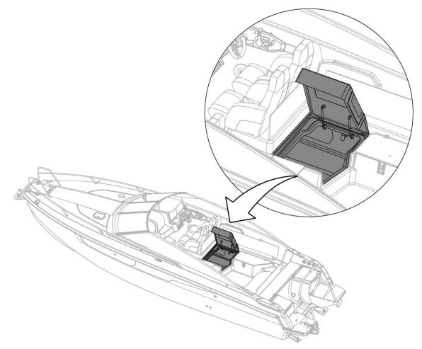
Figure 4.2 Access hatch to mid cabin
