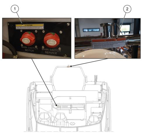
Figure 2.4 Aft deck safety labels
