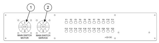
Figure 8.1 Yamarin 88 DC main switches and fuse panel
