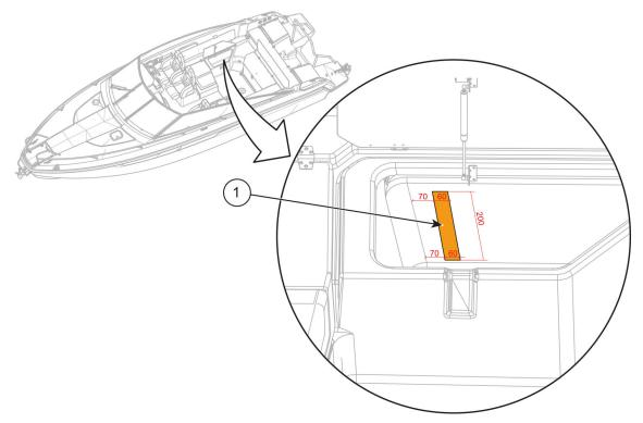
Figure 2.7 Deck seat box fire extinguisher
