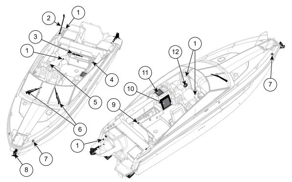
Figure 8.3 Yamarin 88 DC electrical equipment
