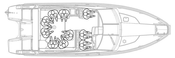
Figure 4.1 Yamarin 88 DC seats for a maximum of ten (10) passengers
