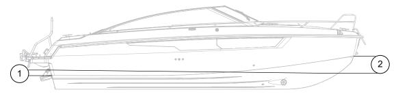
Figure 3.1 Yamarin 88 DC antifouling paint area
